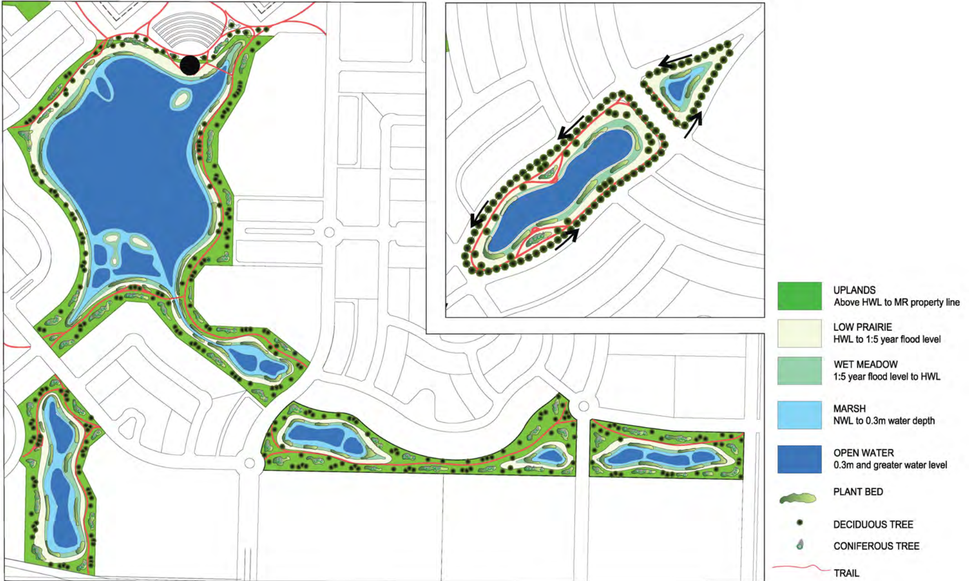
Figure 19: Constructed Wetlands Complex/Stormwater Facility Plan
