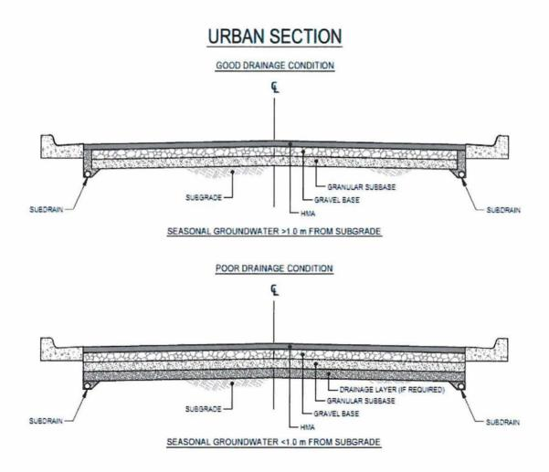
Figure A: Sample Urban Cross Section Drainage Conditions
