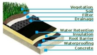
Portland's new design policy requires design and Figure 1.2: The Components of a Green Roof<sup>1</sup> construction of all new city-owned facilities to
