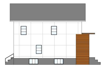
80 square feet of cedar plank is provided along the side building elevation which faces the flanking street. The side elevation facing the flanking street has an area of 840 square feet, requiring the placement of a minimum of 42 square feet of window and/or door area. Five windows are provided resulting in a total window area of 75 square feet.
