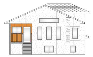
50 square feet of a cedar accent material is provided along the rear elevation of the dwelling which faces a linear park. The rear elevation has an area of 1,100 square feet, requiring the placement of a minimum of 55 square feet of window and/or door area. In this example, 124 square feet of window and door area has been provided.
