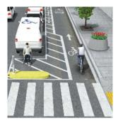
Improvements include a wider parking space to permit adequate space for ramps to be deployed, a buffered connection to an existing curb ramp, and a narrowed bike lane to slow cyclists adjacent to the accessible parking stall.
