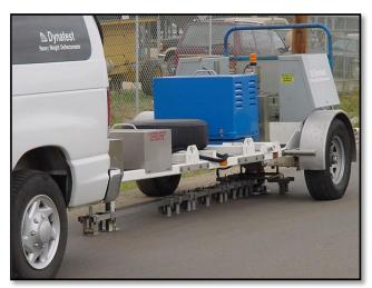
Figure 4: Heavy Weight Deflectometer (HWD)
