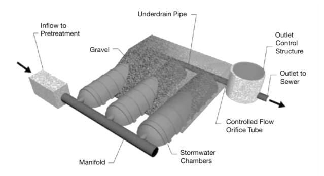
**Orifice** – Usually an orifice provides the control for the permitted release rate from a CW. The preferred minimum diameter is 100 mm, no less than 75 mm, to minimize the occurrence of outlet clogging. Where small orifices are required, consideration should be given to providing an overflow outlet that would operate in the event of blockage of the primary orifice. The orifice plate should be constructed of stainless steel or an approved equivalent.
