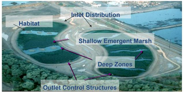
Site conditions frequently constrain the L:W ratio, prompting the use of design techniques to optimize uniform flow distribution through odd shaped sites. Innovative use of habitat islands, shallow zones, or large woody debris flow barriers in addition to deep zones can be used to route water through wetland layouts.
