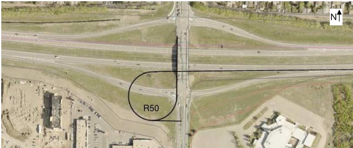
Figure 6.1: Preston Avenue Interchange Option with Loop Ramp
