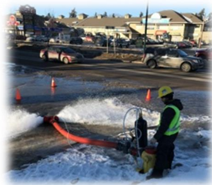
Figure 5.17 - Fire Flow Testing
