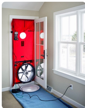
Figure 2: Blower door test
