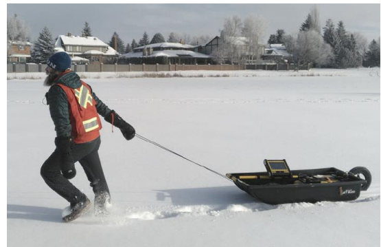
GPR Ice Mapping Courtesy of G3TECH SK LTD.
