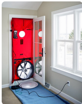
Figure 2: Blower door test
