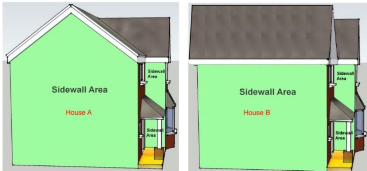
Exhibit 2. Examples of Sidewall Area Calculations.
