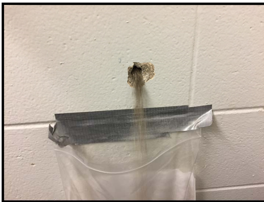
Photograph 2: Asbestos-Containing Vermiculite Insulation.
