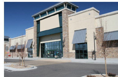
A good example of varied roof heights and changes in wall plane and the use of a variety of canopies and awnings along the front elevation
