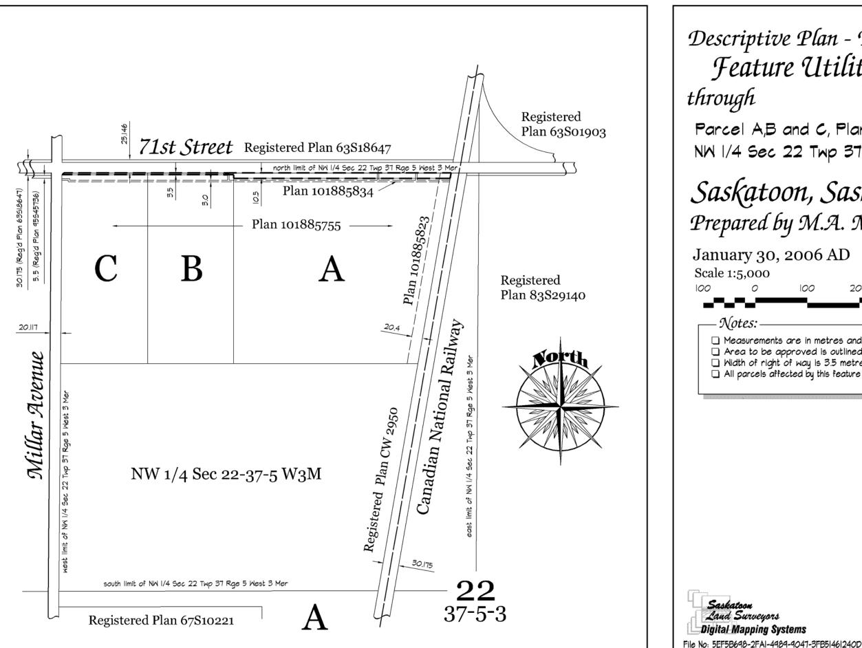
Descriptive Plan - Type II Showing Feature Utility Right of Way Parcel A,B and C, Plan 101885755 NW 1/4 Sec 22 Twp 37 Rge 5 W3M Saskątoon, Saskątchewan Prepared by M.A. Marien S.L.S. 500 100 200 Measurements are in metres and decimals of a metre. Area to be approved is outlined by a heavy dashed line. U Width of right of way is 3.5 metres unless otherwise shown. All parcels affected by this feature have an extension zero unless otherwise shown.
