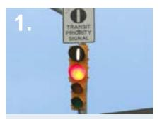
**Transit Signal Priority Measures** use existing traffic signal infrastructure, bus arrival detection and software logic to limit bus delay at traffic signals.
