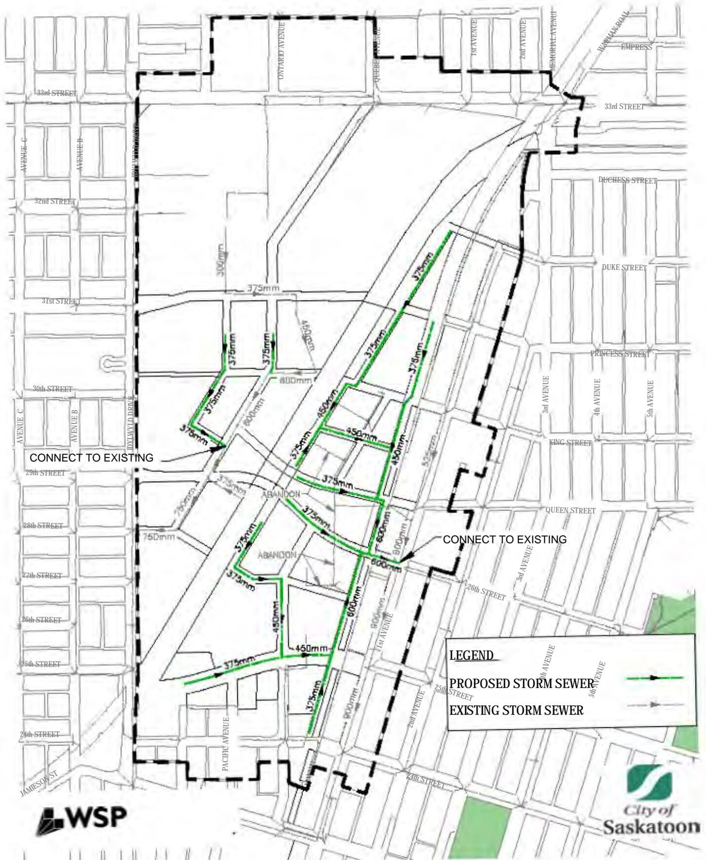
Figure 5.60 - Storm Sewer Concept Plan
