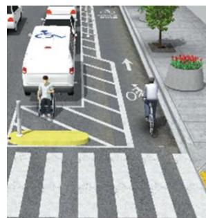
Improvements include a wider parking space to permit adequate space for ramps to be deployed, a buffered connection to an existing curb ramp, and a narrowed bike lane to slow cyclists adjacent to the accessible parking stall.
