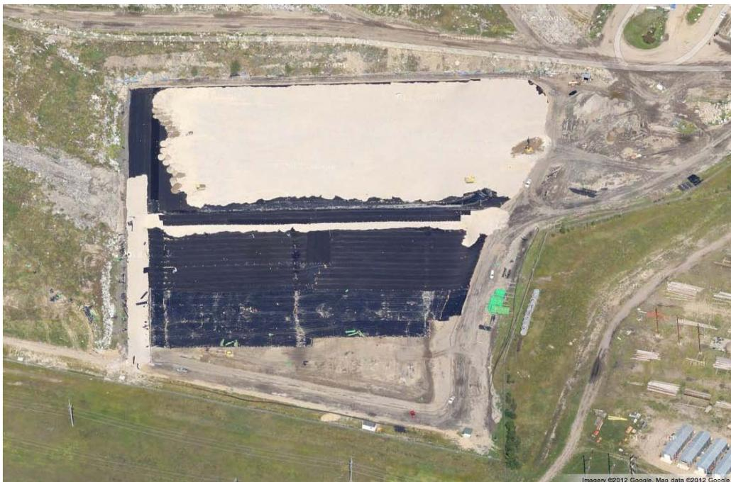
Features include a geosynthetic clay liner, high-density polyethylene geomembrane and non-woven geotextile, drainage layer, leachate collection system, and lift station.
