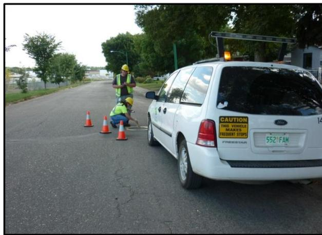
**Figure 3: Manual Condition Rating**
