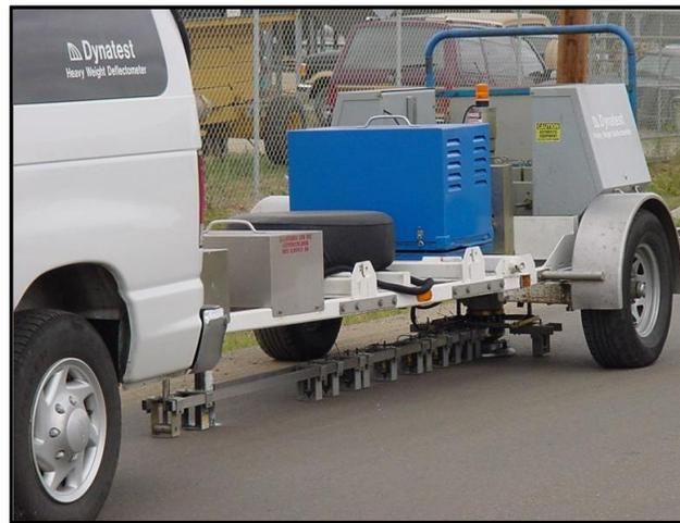
**Figure 4: Heavy Weight Deflectometer (HWD)**
