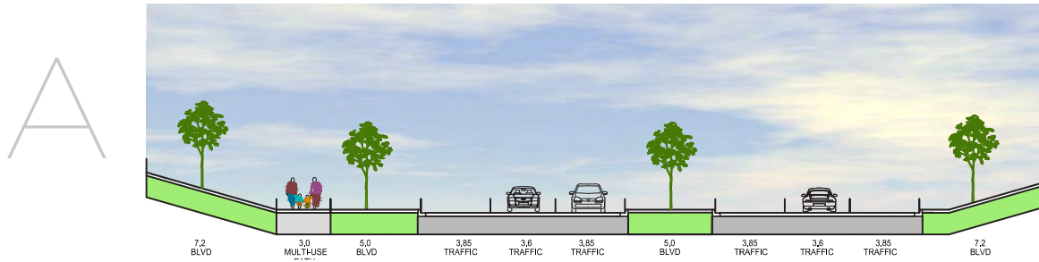
Figure 23: Cross Section A (50.0m ROW)
