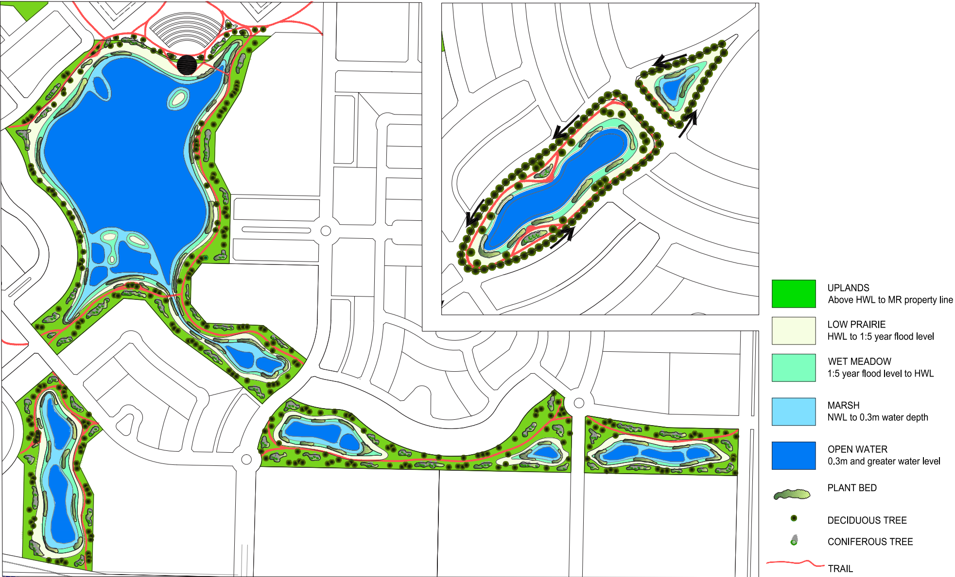
Figure 19: Constructed Wetlands Complex/Stormwater Facility Plan
