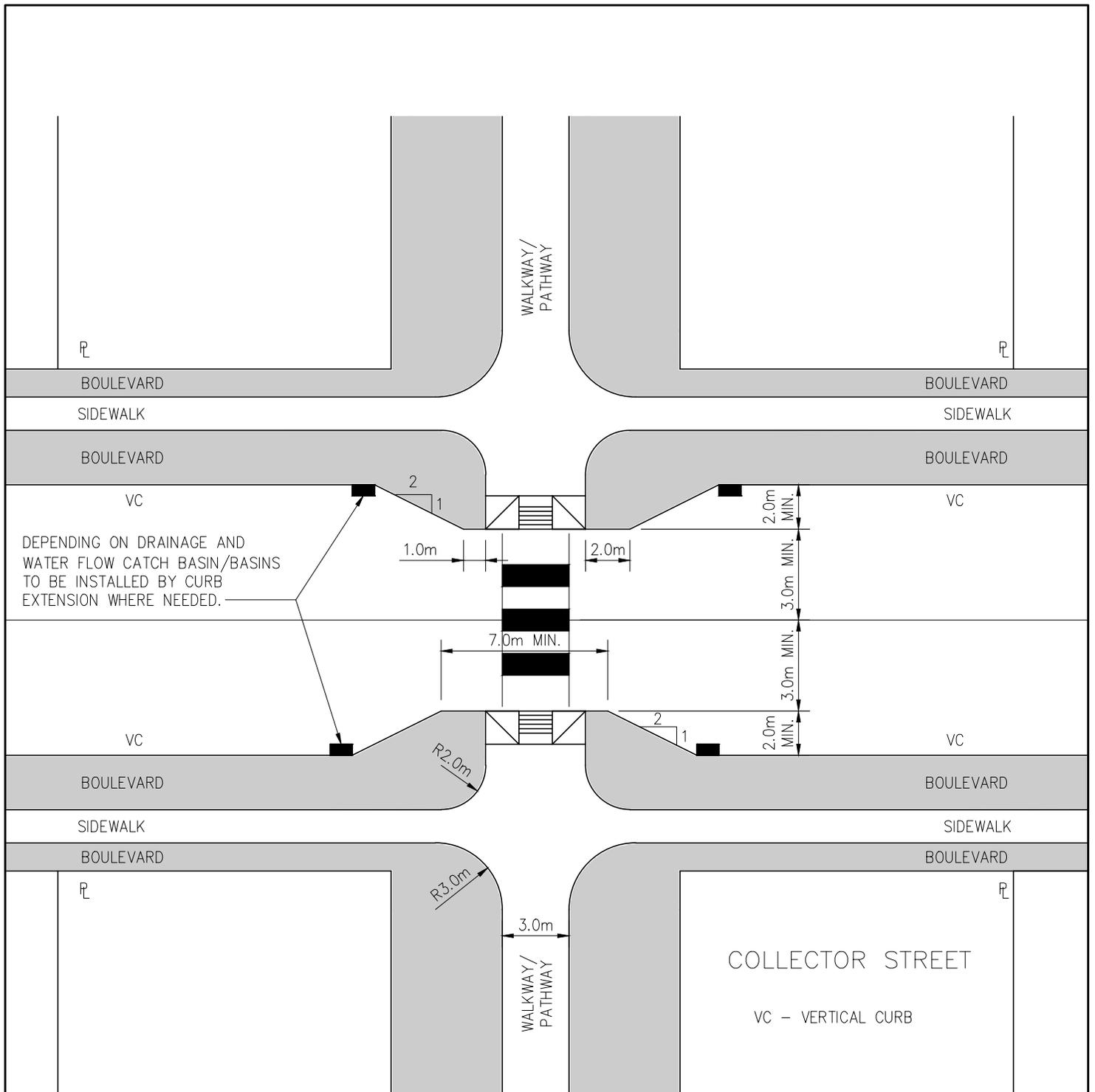
DEPENDENT ON DRAINAGE AND WATER FLOW CATCH BASIN/BASINS TO BE INSTALLED BY CURB EXTENSION WHERE NEEDED.
