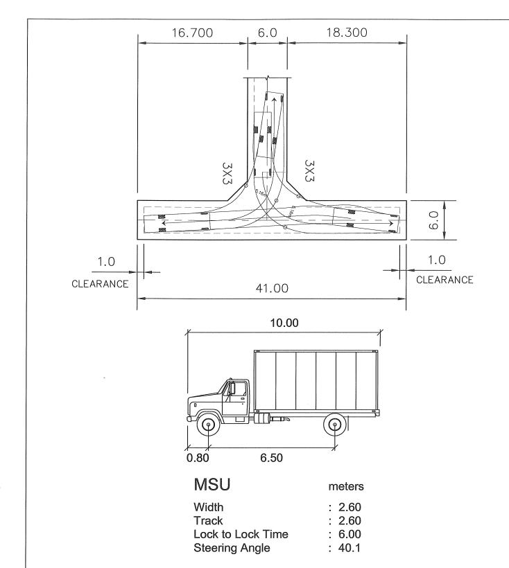
Vd: 1999 TAC (MSU) MEDIUM SINGLE UNIT VEHICLE PATH: ONE STEERING REVERSAL
