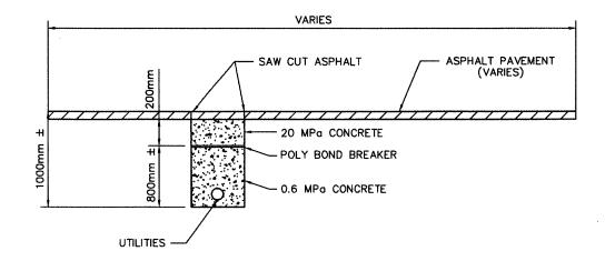
\* ASPHALT SHALL BE PLACED AT 75mm THICK OR MATCH EXISTING THICKNESS WHICHEVER IS GREATER.
