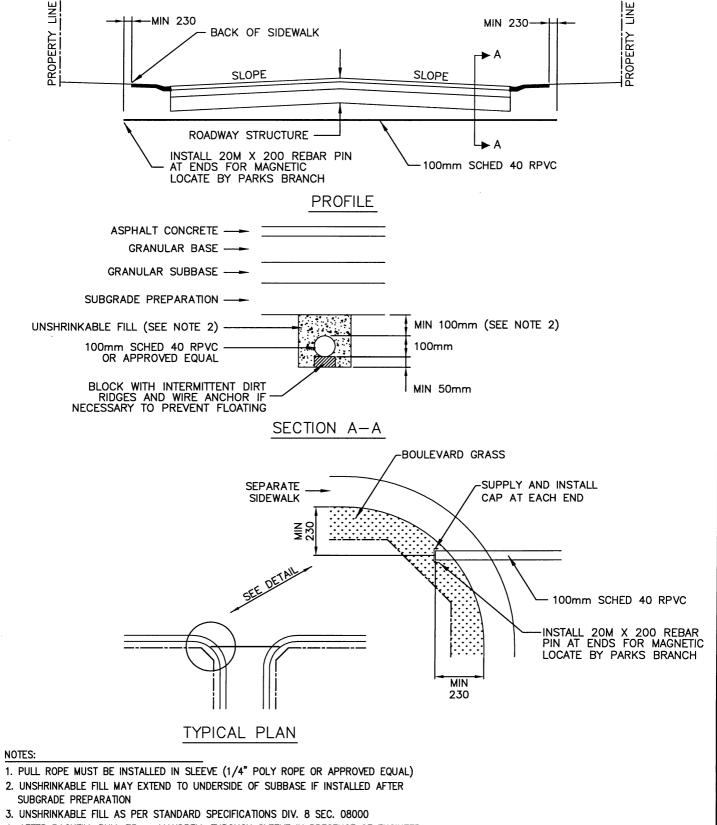
4. AFTER BACKFILL PULL 75mm MANDRELL THROUGH SLEEVE IN PRESENCE OF ENGINEER
