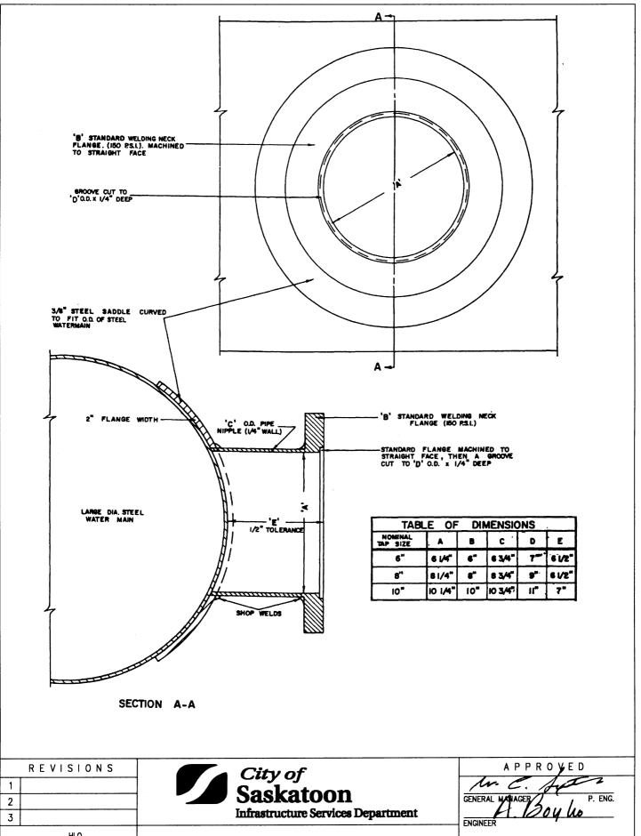
HLO DRAWN BY \_ ENGINEER WELDED TYPE TAPPING SADDLE FOR 06-01-27 DATE \_\_ SCALES : LARGE DIAMETER STEEL WATERMAINS CHECKED BY . PLAN NO. 102-0012-009r001 DATE
