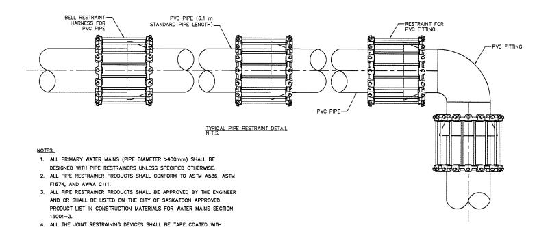
BELL RESTRAINT HARNESS FOR C905 PVC PIPE (OR APPROVED EQUIVALENT)
