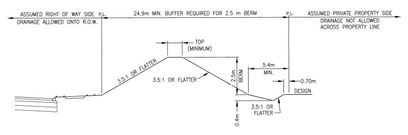
THESE ARE FOR EXAMPLE ONLY; CALCULATE THE BUFFER REQUIREMENT BASED ON THE DESIRED BERM HEIGHT
