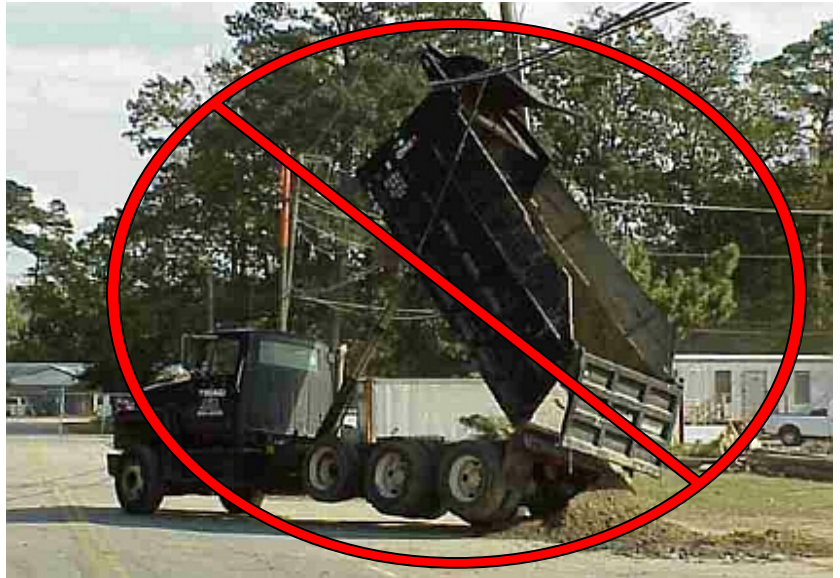
Figure 21 - Truck contacting overhead power lines.
