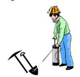
Excess dirt should be cleaned with a wire brush and a rag prior to soaking with disinfectant. Soak items with disinfectant solution (min 5% sodium hypo-chlorite solution), let soak for a minimum of 7 seconds. Scrub item with a clean rag then rinse clean with disinfectant solution. Let tools dry before storing.
