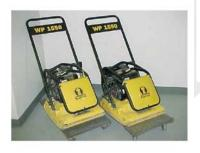
Walk behind vibratory compactor can be used around mains, connections and manhole barrels etc. Backfill shall be placed in 150mm (6inch) lifts.
