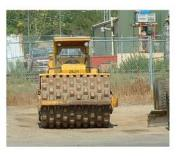
Vibratory Sheep's foot packer must be used for larger excavations. Backfill shall be placed in 150mm (6inch) lifts.
