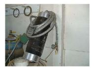
The sewer plug is used to stop flow in the sewer.
