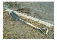
The tunnelling shovel is used for digging around the pipe.
