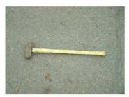
The sledgehammer can be used for knocking the support block into place.
