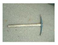
The pickaxe is used to break up hard soil.
