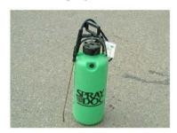
Disinfectant sprayer is used to apply disinfectant (Min 5% Sodium Hypochlorite solution).
