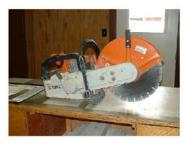
Pipe cutter is used to cut all types of sewer and water pipes.
