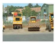
Vibratory roller packer is a compactor used in large excavations.
