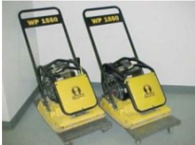
Figure 71 - Walk Behind Vibratory Compactor
