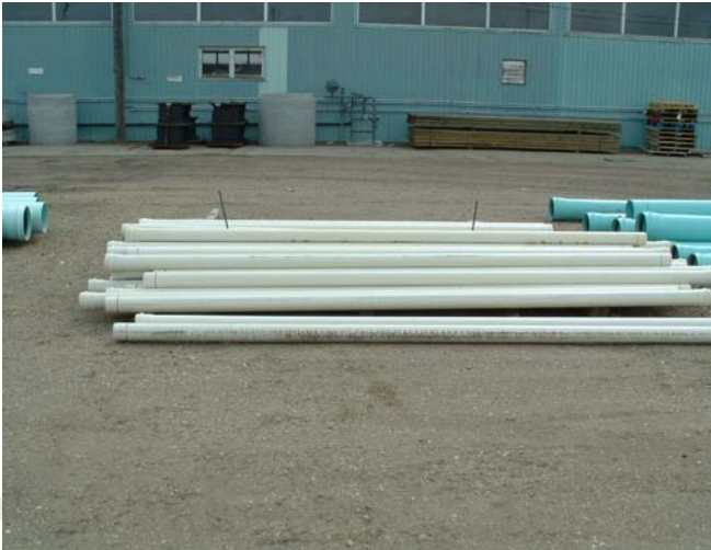
Figure 102 - PVC Sewer Pipes
