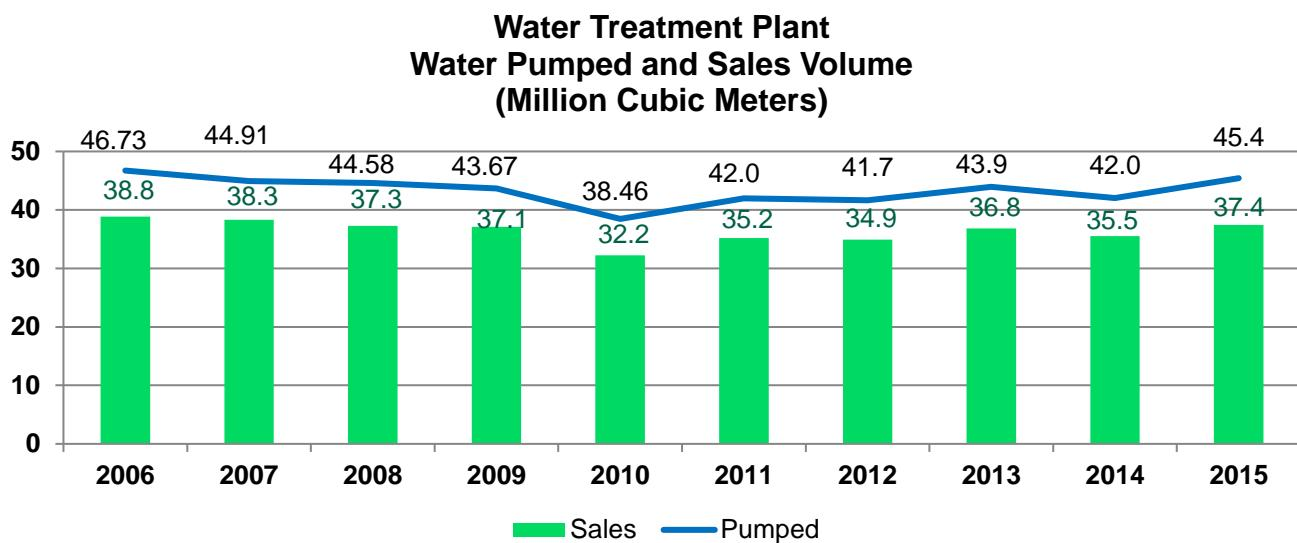
The above chart compares the annual volume of treated water pumped from the WTP into the distribution system and the volume of water sold. Due to a water meter failure, the pumpage was estimated from 2010 to 2013 based on an assumed water leakage rate of 16.2%. In 2015, unmetered water was 17.6% of total water pumpage. The difference between the volume of treated water pumped and sold was due to the following:
