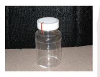
Samples are to be taken for bacterial testing. Use sealed 120 mL plastic bottles with sodium thiosulfate (an agent used to neutralize the chlorine in the water). The bacteria sample bottles cannot be reused as the sodium thiosulfate powder gets washed out.
