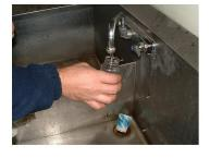
Turn the water stream down to allow filling the sample bottle without having any splashing occur. Let run for 30 sec. then place the bottle under the full stream of water. No water from the stream should be running down the sides of the bottle.
