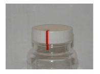
Peel the plastic seal off from around the lid of the bottle. Do not open the bottle until immediately before use. Do not use sample bottles that are not sealed. Do not set the sample bottle lid down while taking the sample.
