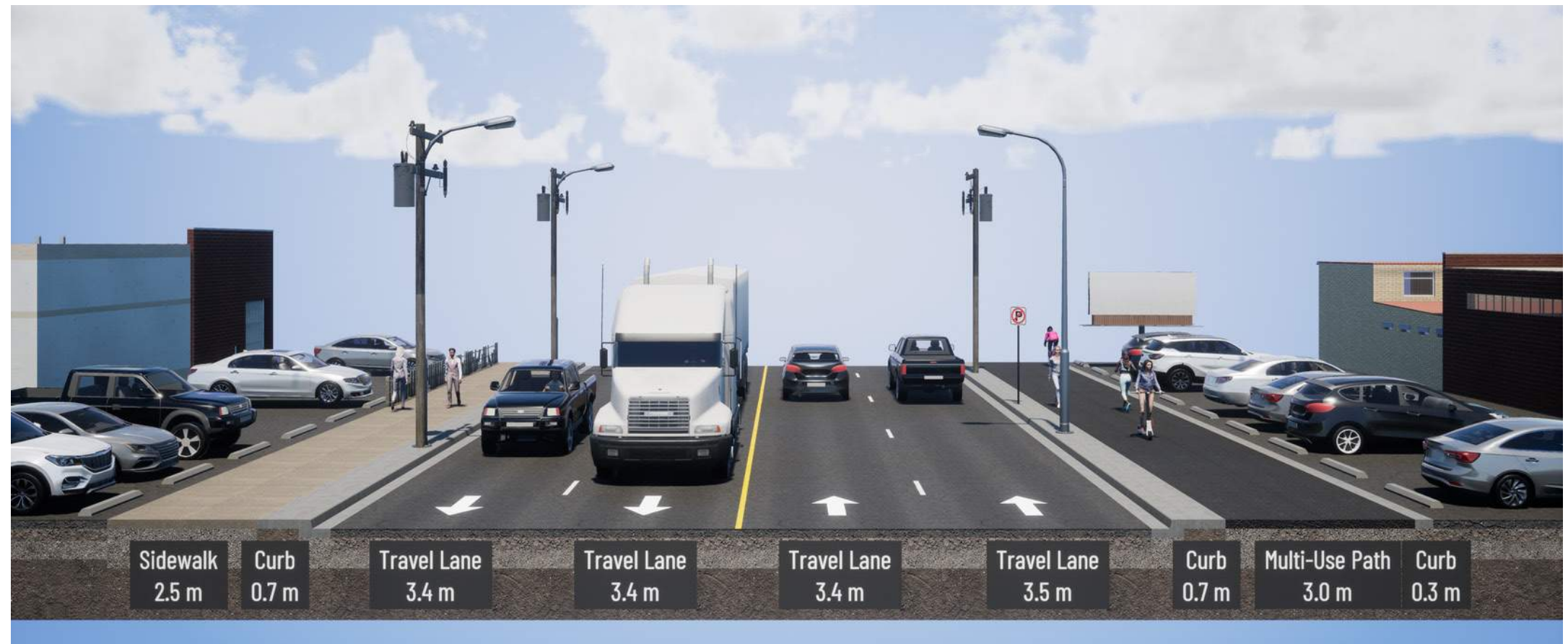
Sample cross section of multi-use pathway on Avenue C. Additional property would be required.
