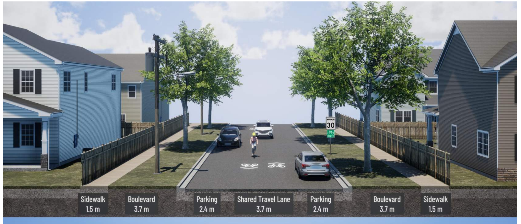
Sample cross section of neighbourhood bikeway on Avenue C. Recommended posted speed 30 km/h pending Council approval.
