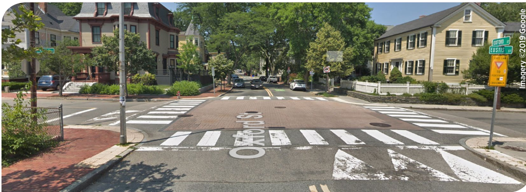
Figure 5.12 Raised intersection with raised crosswalks on Oxford Street in Cambridge, MA
