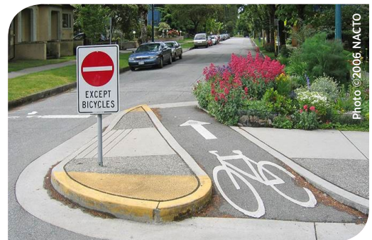
Figure 5.17 - Directional closure in Vancouver, BC
