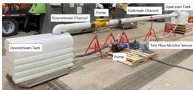
Figure 5.13 - Flow Bench for Equipment Testing and Calibration
