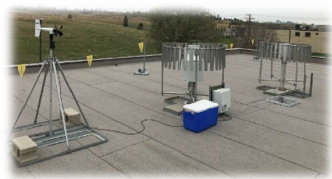
Figure 5.12 - Precipitation and Wind Measurement Station
