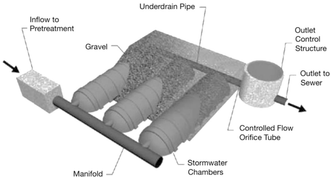
**Orifice** – Usually an orifice provides the control for the permitted release rate from a CW. The preferred minimum diameter is 100 mm, no less than 75 mm, to minimize the occurrence of outlet clogging. Where small orifices are required, consideration should be given to providing an overflow outlet that would operate in the event of blockage of the primary orifice. The orifice plate should be constructed of stainless steel or an approved equivalent.
