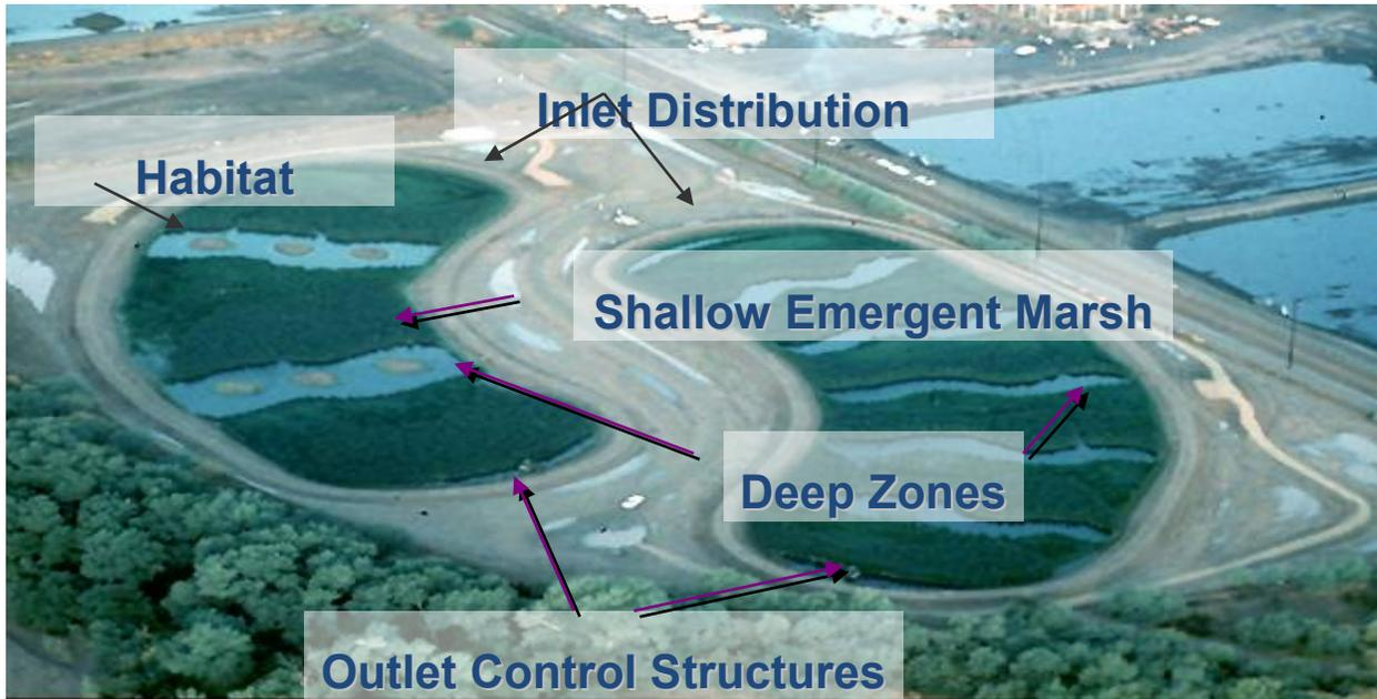
Site conditions frequently constrain the L:W ratio, prompting the use of design techniques to optimize uniform flow distribution through odd shaped sites. Innovative use of habitat islands, shallow zones, or large woody debris flow barriers in addition to deep zones can be used to route water through wetland layouts.
